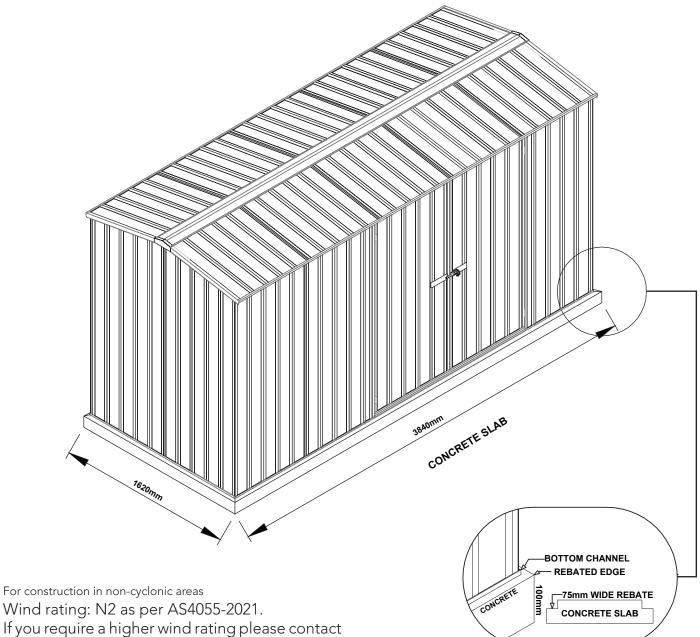
For construction in non-cyclonic areas Wind rating: N2 as per AS4055-2021.
